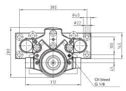
1) Dimensions and weight depend on thickness of brake disk.
