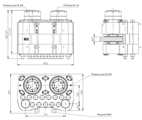
$^{\rm 1)}$  Dimensions and weight depending on thickness of brake disk.
