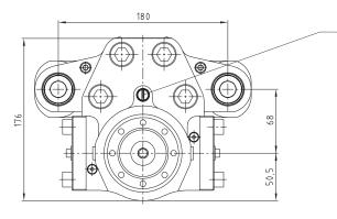
1) Dimensions and weight depend on thickness of brake disk.
